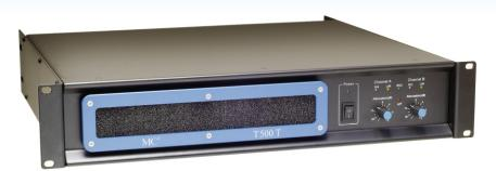
Designed for use in a variety of applications in the 70V/100V fixed installation market, where sonic quality and reliability are the highest priorities, the high performance T500-T & T1000-T use complimentary AB bipolar output stages, combined with the unique MC<sup>2</sup> current driven floating drive stage and conventional analogue level controls.
